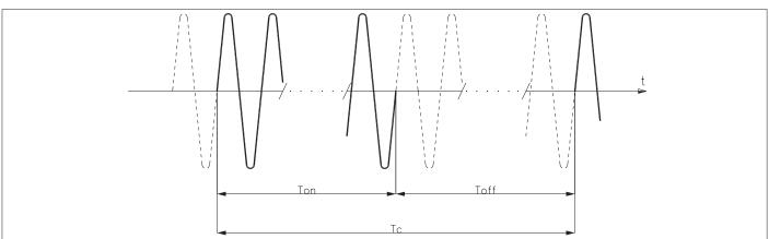
For example, if Tc = 10sec, if the power value is 20% there is conduction for 2 sec (100 conduction cycles @ 50Hz) and non conduction for 8 sec (400 non conduction cycles @ 50Hz).
